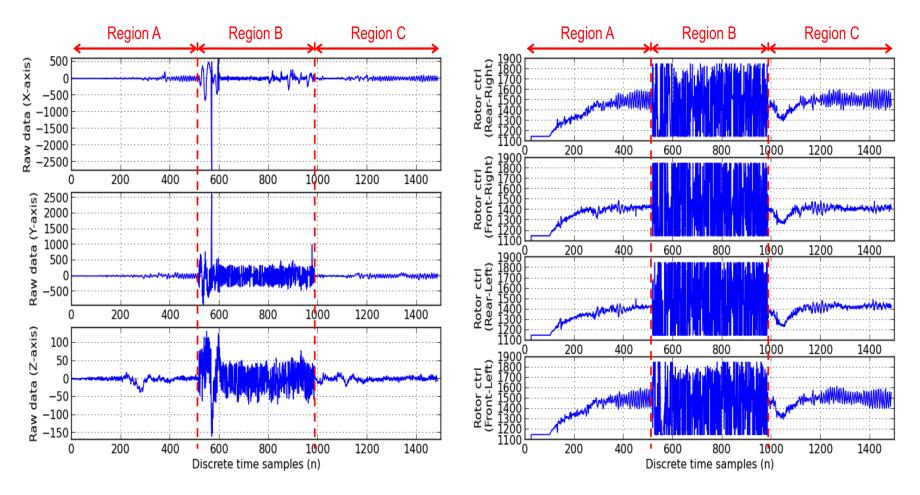
Raw data samples of the gyroscope
